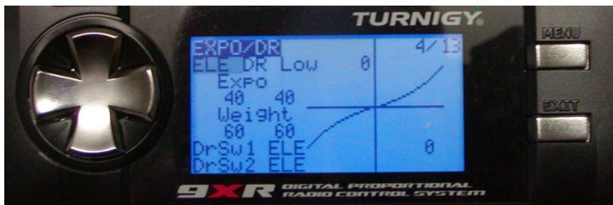
Start by adjusting High rate. Press DOWN to highlight the Expo values and use the LEFT and RIGHT keys to set a fairly conservative expo value such as 25%. Then move DOWN to Weight, which should already be set at 100%. Adjusting this is one way to fine tune the travel (the other way is to use the Limits page 6/13).
