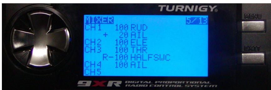
The rudder servo now has 20% movement when the aileron moves 100%. In a turn when you move the aileron stick to bank the aircraft the rudder will move to give a better coordinated turn without the pilot having to move the rudder at all. But when steering on the ground, for example, you still have 100% control of the rudder by using the rudder stick. The plus sign means the two inputs to the rudder channel are added together.
