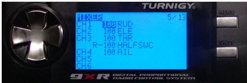
Let's enter an aileron-to-rudder to mix for our Piper Cub. Move the cursor down to highlight RUD. Press Menu. A pop-up screen appears:
