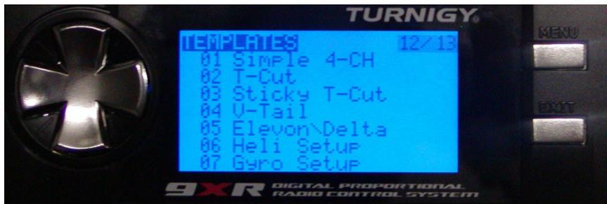
There in Templates 02 and 03 you will see two kinds of throttle cut mix. T-Cut simply enables the THR.CUT switch on the transmitter to disable the throttle stick. Sticky T-Cut goes one step further in safety and requires you to move the throttle stick to Low before the throttle is re-armed.
