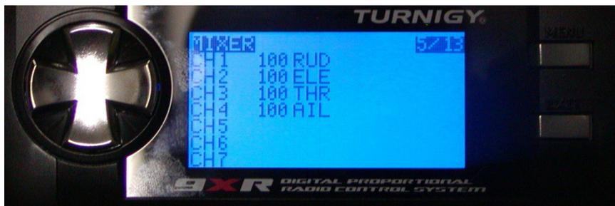
What you will see is the first four channels assigned to the four stick inputs in the order chosen earlier under Radio Setup (here RETA, but yours might be TAER, AETR, etc.). The 100 means that full movement of the stick will produce 100% movement of the corresponding servo.
