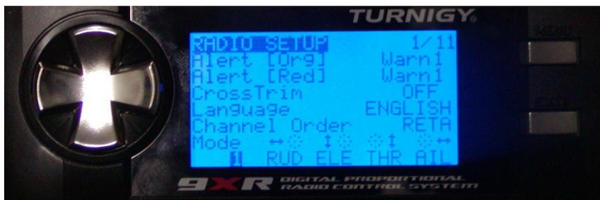
This channel order determines the sequence of controls used throughout the transmitter for setting up and editing all models and the sequence of channels used on your receiver for the connection of your servos. To change it, highlight and use the LEFT and RIGHT keys to select the order you want. For example, modules and receivers using the Spektrum protocol always use the sequence TAER, as their failsafe arrangement requires the use of channel 1 for throttle.
