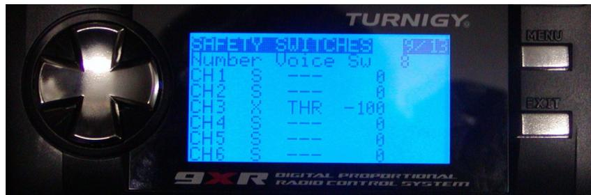
In this case Channel 3 (i.e., the third servo socket on the Rx) is the throttle channel. When the THR switch is positive then the sticky throttle cut is active.
