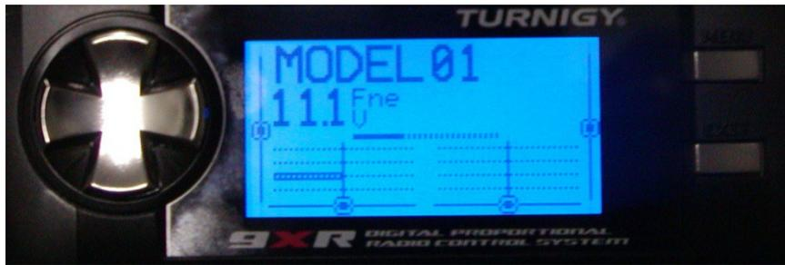
As a first step, we want to get to the Radio Setup and other screens that provide information and enable the adjustment of settings relating to the basic functioning of the transmitter. Press the left side of the cross-shaped navigation button for about half a second. We'll call this LONG LEFT, as opposed to a short press LEFT. You'll soon get used to this very important difference.
