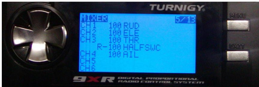
You will see that implementing T-Cut has added an extra mix to the throttle channel. The function of this is to replace the throttle stick input with a full low throttle setting when the THR.CUT switch is activated. (If you want to see what's going on, go to the Mixer screen and look at Channel 14. To understand the logic, you'll need to study *Ersky9x Explained*.)
