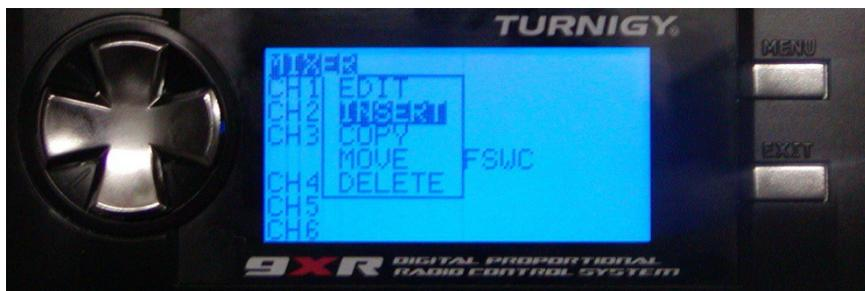
Select INSERT and press MENU. This adds an extra line for the Rudder servo channel that allows it to be controlled by the Aileron stick.
