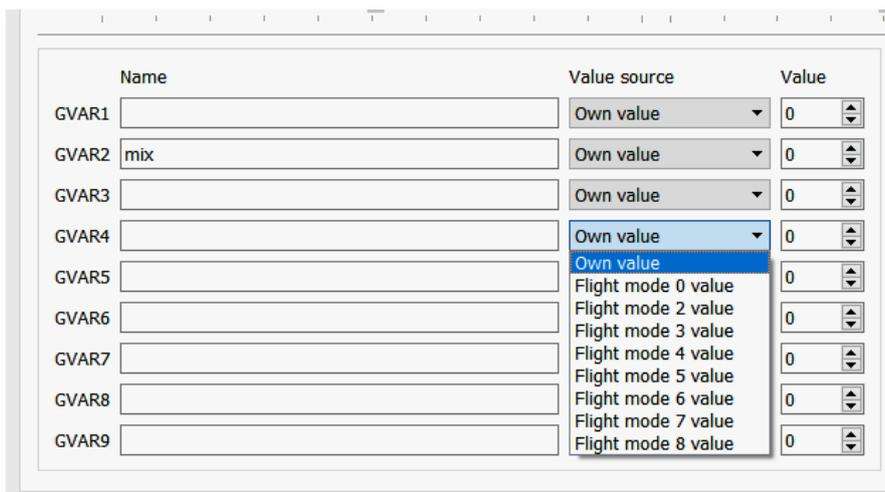
Flight modes 1 to 8 have an extra drop down box, **Own value** available. This box enables the global variable to take the value from any of the other flight modes.
