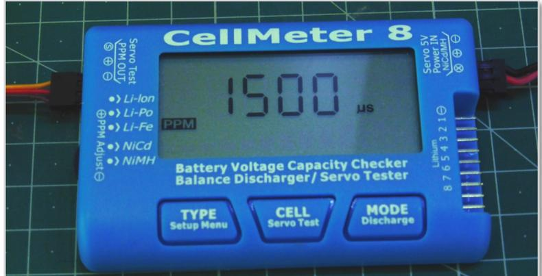
Wherever possible, one should look up the manufacturer’s specifications. Here one can see the operating pulse width extends from 1100µs to 1900µs. This illustrates just how inadvisable it is to use extended limits with some servos and **OpenTX**. One can also see the servo arm travel is ±30°. This is fairly normal and there is a good reason for this.
