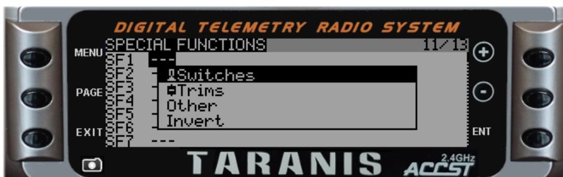
Basically for each **Special Function** there are four parameters, **Switch**, **Action**, **Parameters**, and **Enable**.
