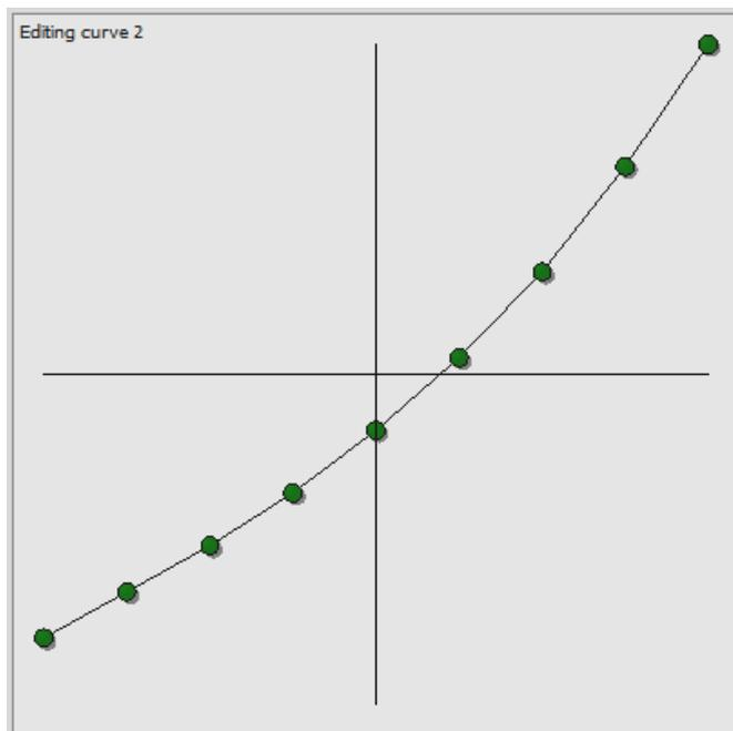
It is possible to also create exponential curves. Here we have an exponential curve which starts at  $-80$  and ends at  $+100$ . Notice there is an extra box in the curve creator, **Coefficient**. This is the exponential value and has been set to 40 here.
