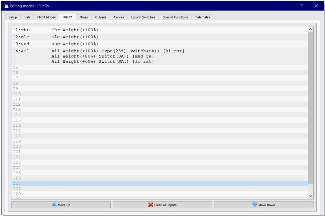
The **Inputs** screen is where the transmitter controls are linked to the inputs that will be manipulated by **OpenTX**. The left hand column shows the inputs defined, highlighted with a capital **I**. The next column shows the actual transmitter controls that are linked to these inputs; in this case the transmitter joysticks. The order of these was defined in the **Setup** screen. Clicking on any line on the **Inputs** screen gives a sub-menu:
