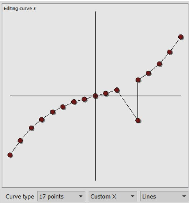
Finally, using the **Custom X** facility, individual points can be moved using the screen cursor to any point between the previous and the next **X** value and to any **Y** value.
