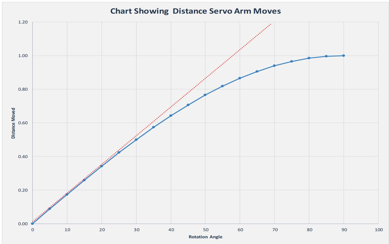
The distance moved is given in terms of the distance from the centre of the servo arm to the linkage hole being used. Thus rotating through  $\pm 30^\circ$ , or a total of  $60^\circ$  will give a good approximation for linear travel, and the servo linkage travel will be half the distance from the servo arm centre to the hole the servo linkage is connected to. Also the sideways movement of the linkage will be minimised.
