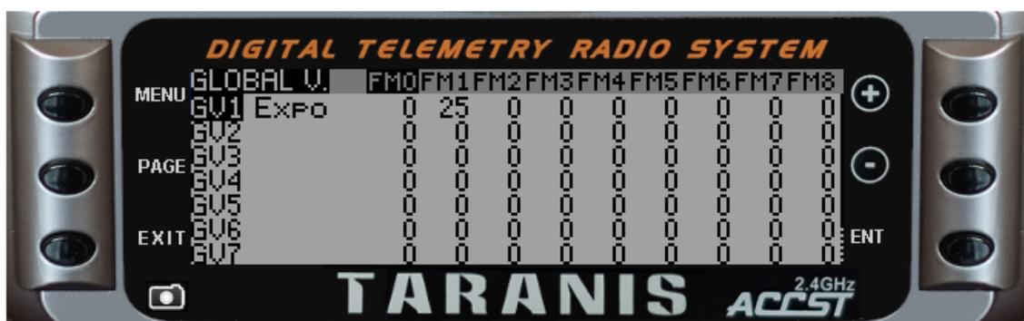
The global variable options differ between flight modes. The following screenshot is using flight mode 0.
