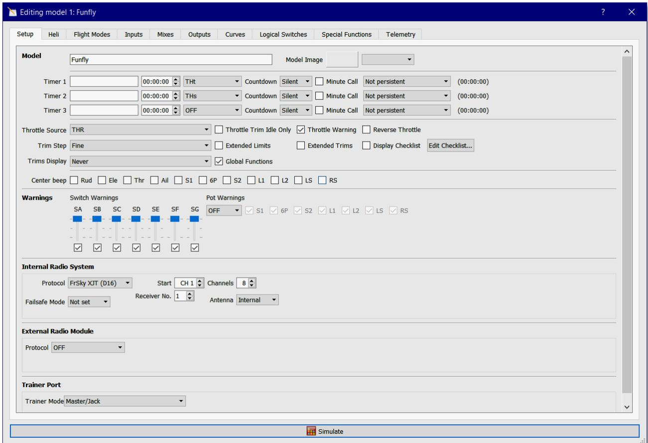
**Model Images** are covered in more detail in the **How-To Part 1** section. Do note that a copy of the model image needs to be on the SD card, and on the mirror image on the computer for the simulator to work correctly. The drop down box on the **Companion** is case sensitive. Using the **radio menu** it is not.
