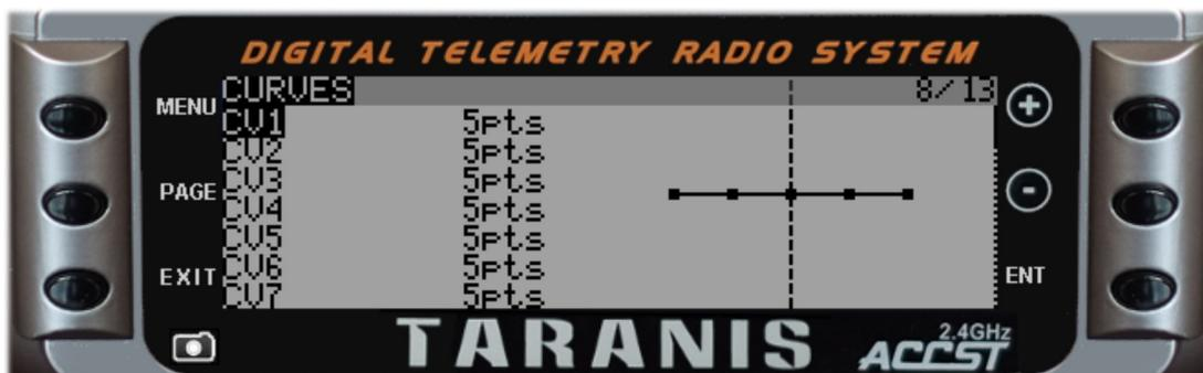
Custom curves can be used either in **Inputs**, **Mixes** or **Outputs**. There are 32 available, and they can have anything from 2 points to 17 points. They can have either fixed or user-definable X coordinates. Curves can be drawn on **OpenTX Companion** using either the mouse and moving points directly, by entering values for each point, or by using the **Curve Creator**.
