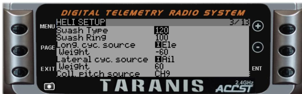
**Note:** The **Noheli** option in the **Radio Profile** must not be ticked, otherwise this heli setup screen will not appear.
