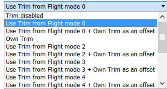
The priority of the flight modes is such as the first FM of 1-8 that has its switch ON is the active one. When none has its switch ON, the default FM0 is active.
