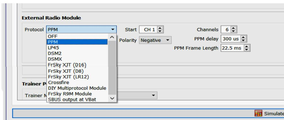
On the FrSky radios, one can also have external radio modules which plug in at the back of the case to talk to other makes of receiver. The module plugs inside the X9E radio. This module can be configured by turning the **Internal Radio Module** off then selecting the appropriate protocol for the external module. The settings available depend on the module type.
