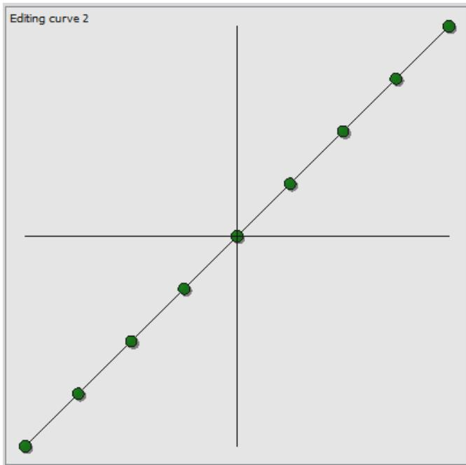
If **Y at X** is reduced to  $-80$  then the curve will completely re-scale to give a curve that starts at  $-80$  and ends at  $+100$ .
