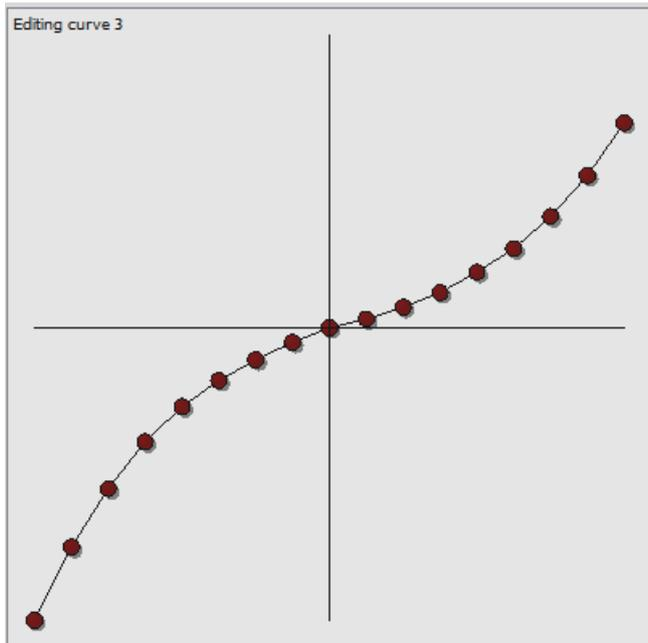
Using the **Side** function, just one side of the curve can be changed. Here the upper limit is reduced to 70, but only for positive values of **X**. Thus there is an easy way of having asymmetrical curves for a variety of purposes.
