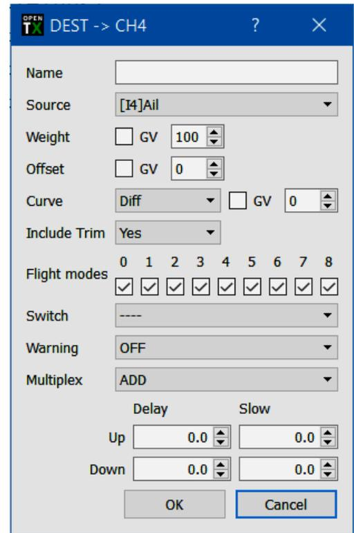
side of the throw) or a curve (built-in or custom) can be assigned. When a custom curve is selected, a press of the **MENU** key will bring you to the curve editor on the transmitter screen.
