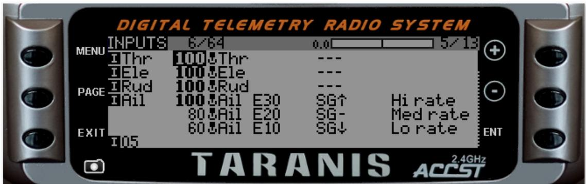
A long press of the ENT button pulls up a series of options including an edit option. This opens up another window with features that match the **Companion** edit window. :
