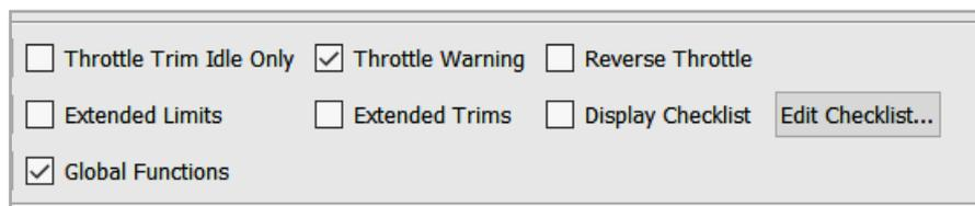
**Throttle Warning** will display a warning when the model is first selected or the transmitter turned on if the throttle is not in the fully minimum setting. This can sometimes come on even if the throttle is fully in the minimum position. If that is the case, then the joysticks need recalibrating.
