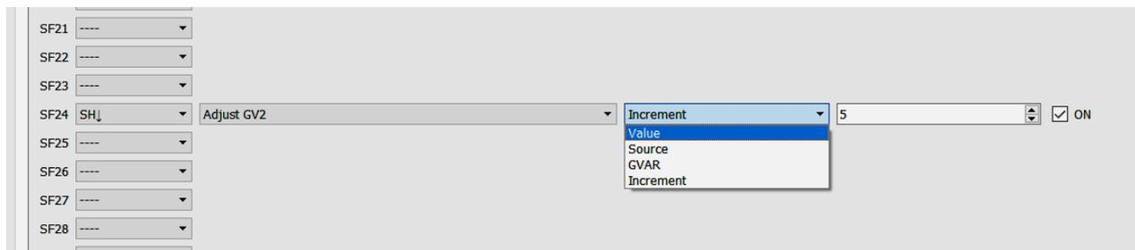
A variety of sources can be chosen. Here momentary switch **H** is used. Then 4 options are given, **Value**, **Source**, **GVAR** or **Increment**.
