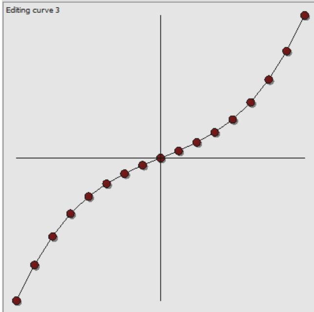
This is a 17 point curve using one of the functions, **Symmetrical  $f(x)=-f(-x)$** .
