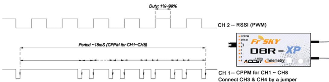
**CPPM channel can not handle all eight channels at the same time with all throws are maxed out, as it does not have enough frame gap. It is recommended to use at most six channels from CPPM channel while leaving off the rest two channels, otherwise improper performance might occur.**
